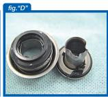
For your customers', families' and friends' uninterrupted driving, please apply adhesive materials by appropriate method and volume. (spread liquid gasket approximately 1.5  $\sim$  2.5mm width uniformly on gasket face only)
