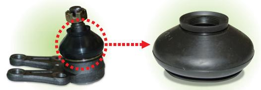
As introduced in our GMB Bulletin #009, the specification for suspension Ball Joint is critical and has a major effect on working life. The function of the Boot is to protect the Ball Stud from foreign materials, such as dirt, mud, thawing salt and so on, that damages operational quality.
