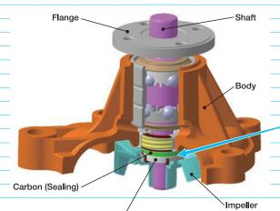
This is due to the sliding surfaces generating a lot of friction before they settle together and benefit from the lubricating properties of the coolant mix which then creates a stable and consistent seal.
